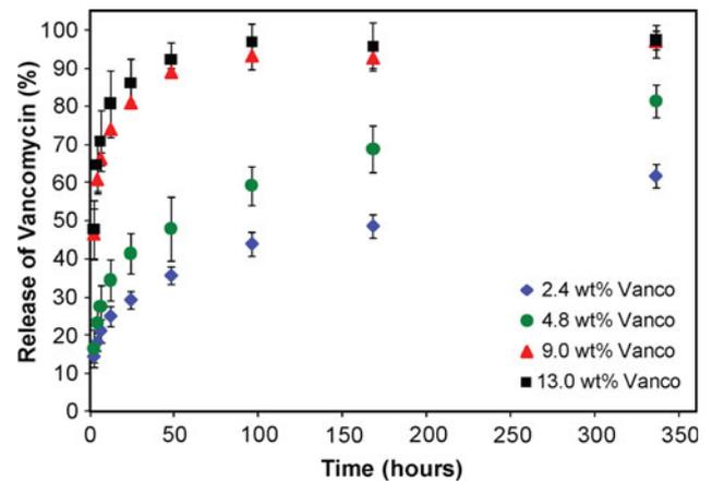
**Fig. 2** A graph shows the release kinetics of vancomycin from pHEMA-nHA-vancomycin composites (Vanco) in PBS (pH 7.4) at 37°C as a function of time and vancomycin encapsulation content. Vancomycin was released in a sustained and dose-dependent manner.
