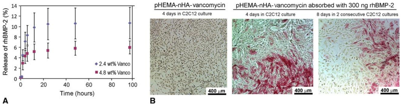
**Fig. 4A–B** (A) A graph shows the release kinetics of rhBMP-2 from pHEMA-nHA-vancomycin as determined by ELISA. After an initial release of 5% and 10% from the 4.8- and 2.4-wt% vancomycin composites (Vanco) in the first 12 hours, respectively, rhBMP-2 release plateaued ( $> 89\%$  retained on 2.4-wt% composites by 24 hours,  $> 94\%$  retained on 4.8-wt% composites by 48 hours). (B) Images (original magnification,  $\times 100$ ) show ALP staining of
