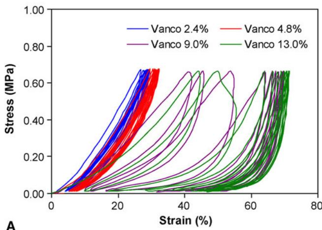
**Fig. 1A–B** (A) A graph shows the compressive stress-strain curves of pHEMA-nHA-vancomycin composites (Vanco) as a function of vancomycin encapsulation content. Ten continuous loading-unloading cycles (from 0.03 N to 10.0 N and back to 0.03 N, loading rate of 3.0 N/minute) were applied to the composite at 37°C in PBS (pH 7.4), using a submersion compressive fixture. The content of vancomycin had a direct impact on the compressive behavior of the composite,
