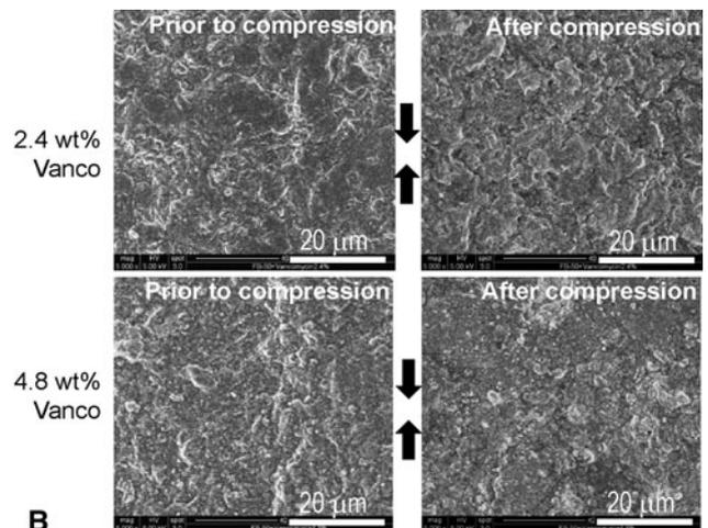
with the stiffness of the composites inversely correlated with the vancomycin content. (B) SEM micrographs (original magnification,  $\times 5000$ ) show cross sections of pHEMA-nHA-vancomycin composites containing 2.4 wt% vancomycin before (left) and after (right) the repetitive compressive loadings. The composites did not reveal any microfractures after the loadings.
